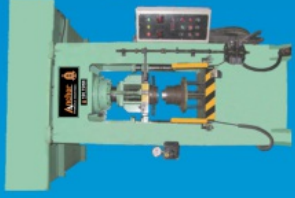
100 TONS DIE CUSHION TYPE DEEP DRAWING PRESS
